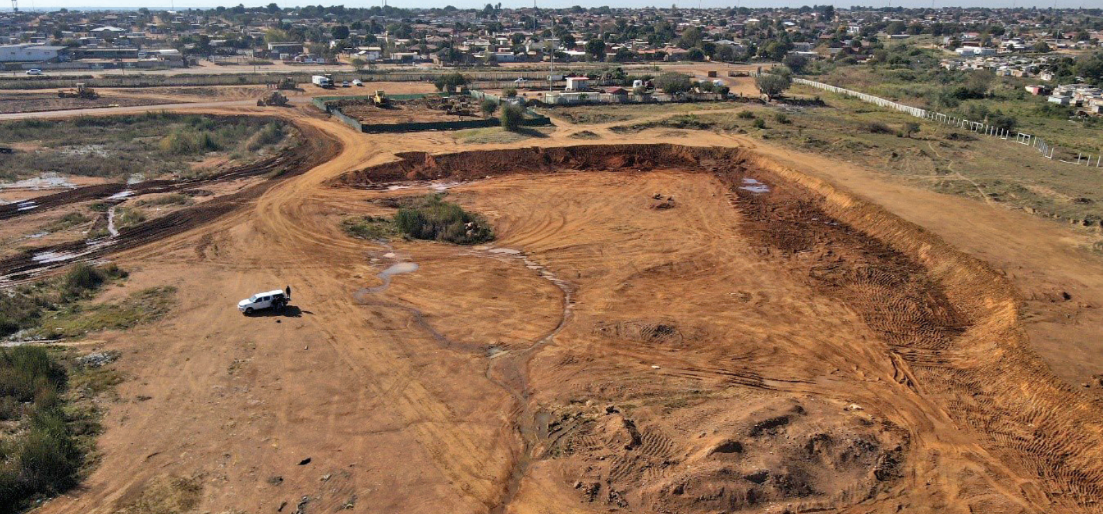
An aerial view of a wet weather cell of a landfill site
